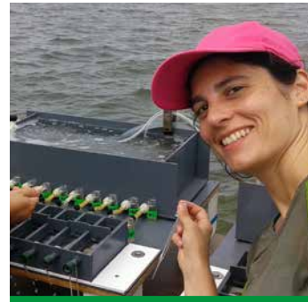
Dr. Galimany uses a tool she designed to measure bivalve filtration in the field.
